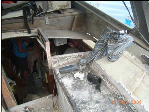
The hole in the bulkhead, the inside of the boat is full of rusty metal
