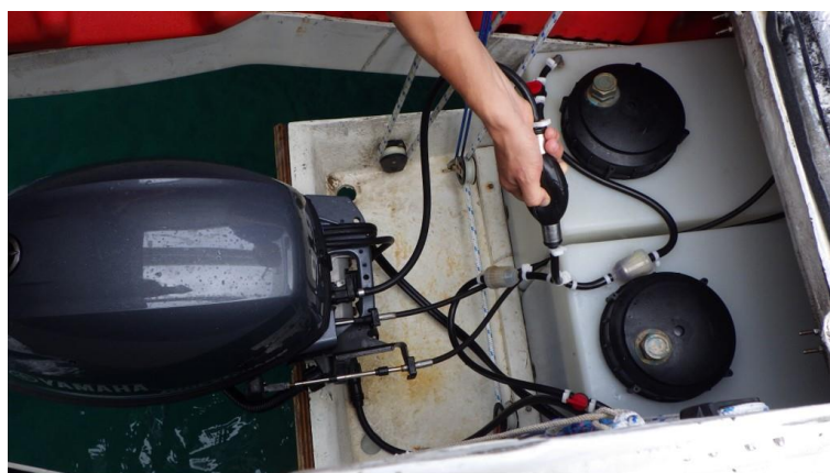
The large tanks can be easily filled from cans using a jiggle pump
