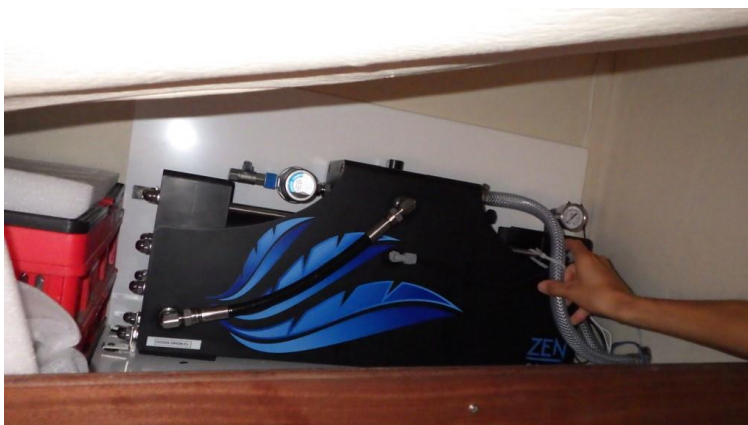
The compact energy recovery watermaker sits on a shelf in the foc'sle
